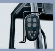
he new efficiency lighting system mploys LED illuminant and new type effector to reduce energy consumption, nprove significantly illumination erformance and prolong work time
